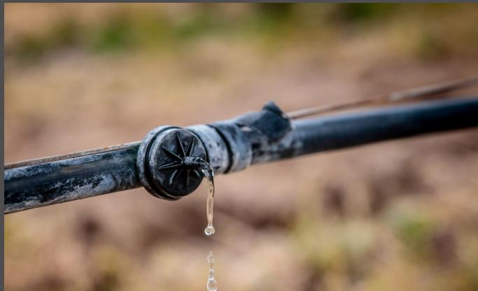
Drip emitter with calcium carbonate scale buildup, suggesting the emitter is plugging.
